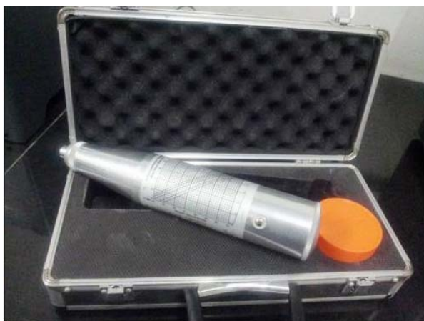
Fig. 2.1: Rebound hammer apparatus
